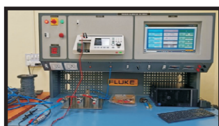
Laboratory Calibrator 0 to 10 bar with 0.01% accuracy
